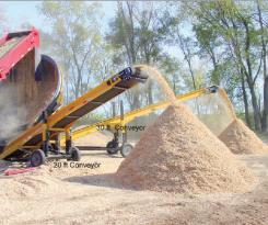
Modular Design Allows for Adding 20', 30' or 40' Conveyors
